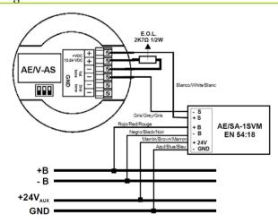
The AE / SA-1SVM module must be installed inside the equipment whose signal must be controlled, or in a box arranged for this purpose. A module can control 1 or more fire alarm devices connected in the same loop. The end of line resistor must be connected to the last connected fire alarm device.
